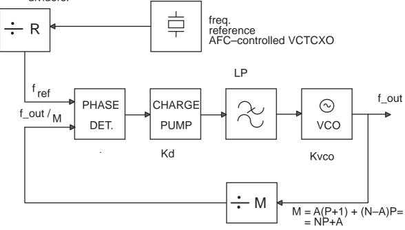
LO–signal is generated by SHF VCO module. VCO has double frequency in DCS1800 and x 4 frequency in EGSM compared to actual RF channel frequency. LO signal is divided by two or four in HAGAR (depending on system mode).
